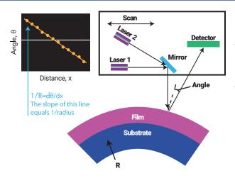
FLX stress measurement systems use the laser lever technique to measure changes in pre and post de-position surface radii and then correlates these measurements into a stress value.
