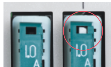
Fuse blowout indication
